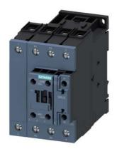
Power contactor, AC-3 40 A, 18.5 kW / 400 V 2 NO + 2 NC 230 V AC, 50 Hz 4-pole size S2 screw terminals 1 NO + 1 NC integrated
