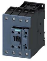
Contactor, AC-3, 50 A/22 kW/400 V, S2, 4-pole, 20-33 V AC/DC, with varistor, 1 NO+1 NC, screw terminal
