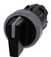
Selector switch, illuminable, 22 mm, round, plastic with metal front ring, black, selector switch, short, 3 switch positions I-O-II, latching, actuating angle 2x45°, 10:30h/12h/13:30h
