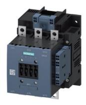
power contactor, AC-3 150 A, 75 kW / 400 V AC (50-60 Hz) / DC operation 110-127 V AC/DC auxiliary contacts 2 NO + 2 NC 3-pole, frame size S6 busbar connections drive: conventional spring-loaded terminal
