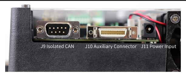
Controller input power supply input utilizes a CUI® PJ-102AH barrel jack connector.
