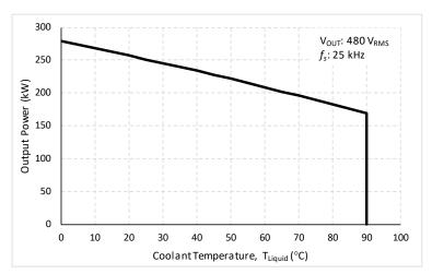
Figure 1. Output Power vs. Coolant Temperature
