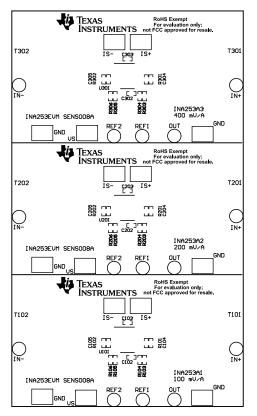
Figure 3. PCB Top Overlay
