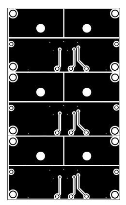
Figure 5. PCB Bottom Layer
