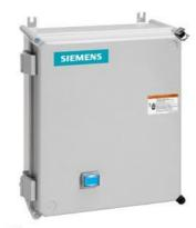
Non-reversing motor starter, Size 3, Three phase full voltage, Solid-state overload relay, OLR amp range 25-100A, Non-combination type, Enclosure type 4X fiberglass, Water/dust tight noncorrosive, Standard width enclosure
