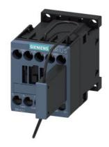
Contactor relay railway, 2 NO + 1 NC 220 V DC, 0.7  $\dots$  1.25\* US, with integrated suppressor diode, Size S00, screw terminal installation on standard mounting rail optimized (20 G) suitable for PLC outputs
