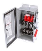
Siemens Low Voltage Circuit Protection Heavy Duty Safety Switches. Type: ENCLOSED, SAFETY SWITCH Std: UL V. Rating: 600V A. Rating: 100A Wattage: 3W No. Of Poles: 3P F. Rating: 60Hz Action: SINGLE THROW Material: 304SS Enclosure: TYPE 12. 2-3 point mounting holes. Insulation: YES O. Cycles: 10000 O. Temperature: (-20F-120F) AMBIENT TEMPERATURE Environmental Conditions: INDUSTRIAL
