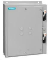
Duplex starter w/o alternator, Size 4, Three phase full voltage, Amb. compensate bimetal OLR, Contactor amp rating 135A, 110V 50Hz / 120V 60Hz coil, Combination type, Two 150A circuit breakers, Enclosure NEMA type 1, Indoor general purpose use
