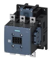
Contactor, AC-1, 400 A/690 V/40  $^{\circ}$ C, S10, 3-pole, 96-127 V AC/DC, PLC-IN optional, with varistor, 2 NO+2 NC, Connection rail/ screw terminal
