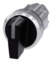
Illuminable selector switch, 22 mm, round, metal shiny, black, Selector switch short, 3 switch positions I-O<II, left latching, right momentary contact type, actuating angle 2x45°, 10:30h/12h/13:30h
