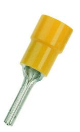
Crimp lug, Pin shape acc. to DIN 46231, Length: 25.5 mm, Max. wire cross-section: 6 mm², Colour: Yellow
