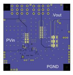
Figure 51b: IRDC3846 Demo board Layout Considerations - Bottom Layer
