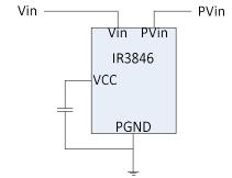
Figure 17: Internally Biased Configuration
