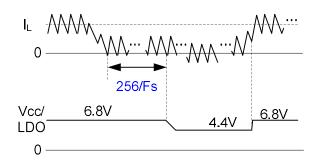
Figure 16: Time Diagram for Smart LDO
