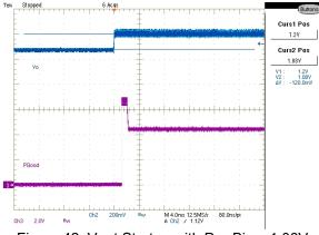
Figure 42: Vout Startup with Pre-Bias, 1.08V Ch2:Vout, CH3:PGood
