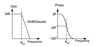
Figure 34: Gain and Phase of LC filter
