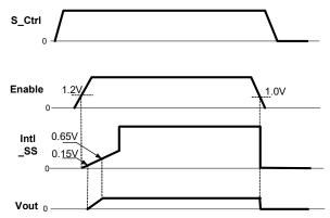
Figure 29: Timing Diagram for Enable controlled Soft-Start / Shutdown
