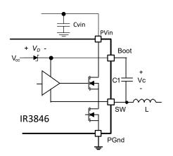
Figure 33: Bootstrap circuit to generate Vc voltage
