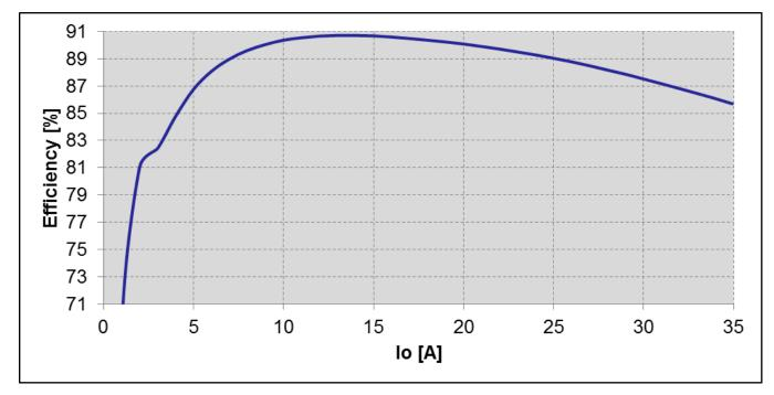
Figure 49: Efficiency versus load current
