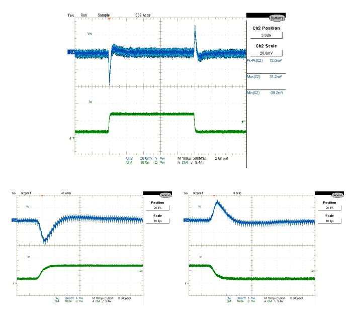
Figure 46: Vout Transient Response, 3.5A to 14.0A step at 2.5A/uSec CH2:Vout, CH4:lout
