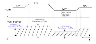
Figure 15: Timing Diagram for Feed-Forward (F.F.) Function
