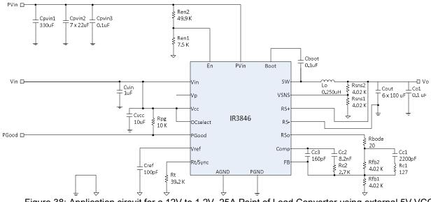
Figure 38: Application circuit for a 12V to 1.2V, 25A Point of Load Converter using external 5V VCC
