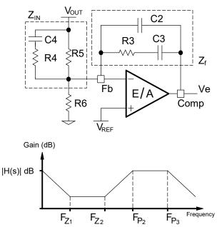
Figure 36: Type III Compensation network and its asymptotic gain plot
