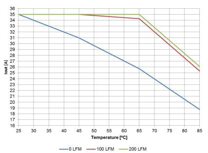
Vin=PVin=12V, Vout =3.3V, VCC=internal LDO (6.8V), Fs = 600kHz
