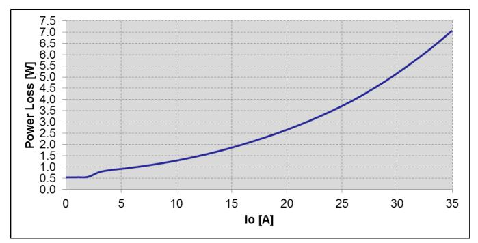
Figure 50: Power Loss versus load current
