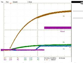
Figure 40: Startup with full load, Enable Signal CH1:Vin, CH2:Vout, CH3:PGood, CH4:Enable
