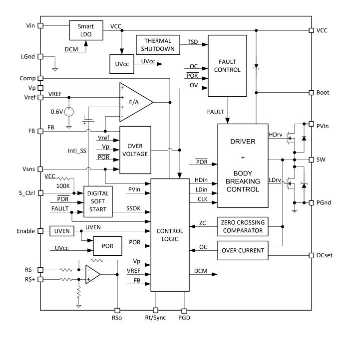
Figure 3: IR3846 Simplified Block Diagram
