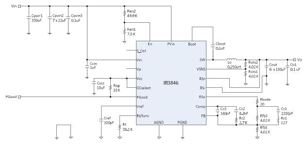
Figure 37: Application circuit for a 12V to 1.2V, 35A Point of Load Converter Using the Internal LDO
