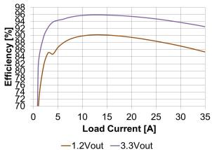
Figure 2: Efficiency [Vin=12V, Fsw=600kHz]
