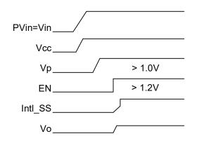
Figure 5: Recommended startup for Normal operation
