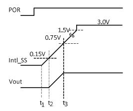
Figure 10: Theoretical operation waveforms during soft-start (non tracking / non sequencing)
