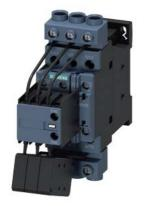
Capacitor contactor, AC-6b 33 kVAr, / 400 V 1 NO + 2 NC, 24 V AC, 50/60 Hz 3-pole, Size S0 screw terminal
