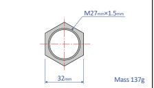
Note: When attaching, make sure that the side without a bearing chamfer is the impact surface.
