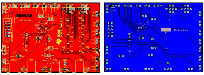
Figure 3. Top Assembly Layer
