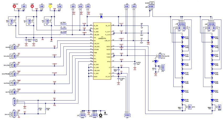
Figure 9. LM3632EVM Schematic
