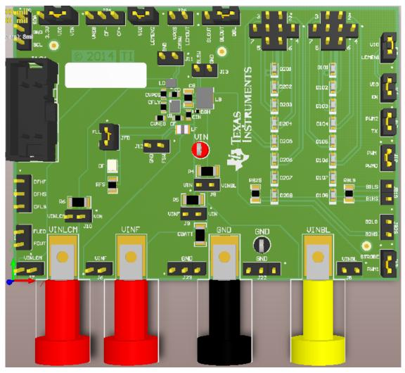
Figure 2. LM3632EVM Recommended Jumper Placement
