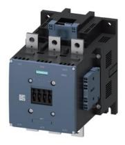
power contactor, AC-3 500 A, 250 kW / 400 V AC (50-60 Hz) / DC 96-127 V AC/DC auxiliary contacts 2 NO + 2 NC 3-pole, frame size S12 busbar connections drive: electronic with PLC interface 24 V DC spring-loaded terminal
