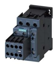
Power contactor, AC-3 9 A, 4 kW / 400 V 2 NO + 2 NC, 110 V AC 50 / 60 Hz, 3-pole, Size S0, screw terminal Removable auxiliary switch
