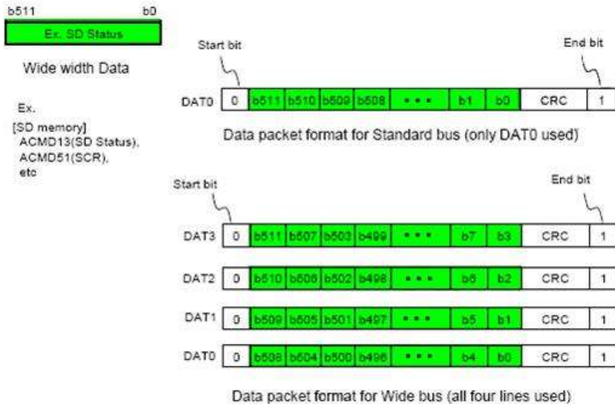
Figure 6-1-7: Data packet format - Wide width data
