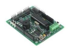
The BotBoarduino is an Arduino Duemilanove compatible microcontroller made specifically for the Lynxmotion robots. It's perfect for controlling your small robotic projects. You can store and run programs independently of a computer. You can also hook up the BotBoarduino to a PS2 controller for remote control of your robotic creation.
