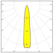
Dimensions: 111.0 mm x 111.0 mm Height: 80.00 mm ~11° spot beam
