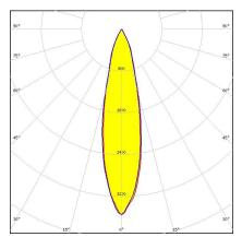
Dimensions: 111.0 mm x 111.0 mm Height: 80.00 mm ~20° medium beam
