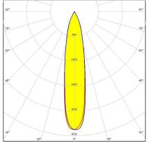
Dimensions: 111.0 mm x 111.0 mm Height: 80.00 mm ~18° smooth spot beam
