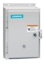
Reversing motor starter, Size 1, Three phase full voltage, Solid-state overload relay, OLR amp range 5.5-22A, 110V 50Hz / 120V 60Hz coil, Non-combination type, Enclosure type 12, Dust/drip proof for indoors, Standard width enclosure
