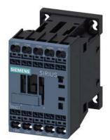
Coupling contactor relay railway 2 NO + 2 NC, DC 72 V, 0.7 ... 1.25\* US, with varistor integrated, Size S00, Spring-type terminal
