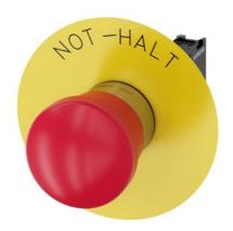
EMERGENCY STOP mushroom-type actuator, 22 mm, round, metal, shiny, red, 40 mm, positive latching, according to EN ISO 13850, pull-to-unlatch mechanism, with yellow backing plate, inscription: NOT-HALT, with holder, 1 NC, screw terminal
