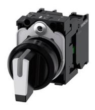
Selector switch, illuminable, 22 mm, round, plastic, white, selector switch, short, 3 switch positions I>O<II, momentary contact type, 10:30h/12h/13:30h, with holder, 1 NO, 1 NO, screw terminal, with laser labeling, upper case and lower case, always upper case at beginning of line
