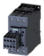
Power contactor, AC-3 65 A, 30 kW / 400 V 2 NO + 2 NC, 24 V AC, 50/60 Hz, 3-pole, size S2 screw terminals
