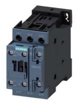
power contactor, AC-3 25 A, 11 kW / 400 V 1 NO + 1 NC, AC (50-60 Hz) DC operation 21-28 V AC/DC, 3-pole, Size S0, screw terminal
