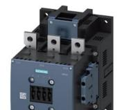
power contactor, AC-3 225 A, 110 kW / 400 V AC (50-60 Hz) / DC operation 23-26 V AC/DC auxiliary contacts 2 NO + 2 NC 3-pole, frame size S10 busbar connections drive: conventional screw terminal auxiliary switch block 2 NO + 2 NC lateral, left + right captive auxiliary switch block, DIN 50012
