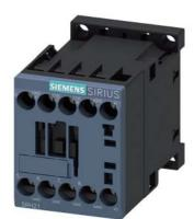
Contactor relay, 2 NO + 2 NC, 277 V AC, 60 Hz, Size S00, screw terminal
