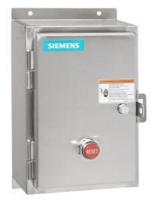
Non-reversing motor starter, Size 2 1/2, Three phase full voltage, Amb. compensate bimetal OLR, Contactor amp rating 60A, 24VAC 50-60Hz coil, Non-combination type, Encl. type 4X 304 S. Steel, Water/dust tight noncorrosive
