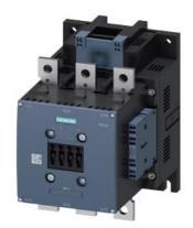
power contactor, AC-3 225 A, 110 kW / 400 V AC (50-60 Hz) / DC operation 200-220 V AC/DC auxiliary contacts 2 NO + 2 NC 3-pole, frame size S10 busbar connections drive: conventional spring-loaded terminal
