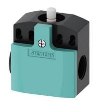
Position switch with increased corrosion protection Plastic enclosure wide, according to EN 50047, 50 mm Device connection 2 x (M20 x 1.5) 2 NO/1 NC slow-action contacts Teflon plunger
