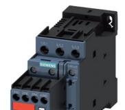
Power contactor, AC-3 9 A, 4 kW / 400 V 2 NO + 2 NC, 24 V DC with plugged-in diode combination, 3-pole Size S0, Screw terminal Captive auxiliary switch
