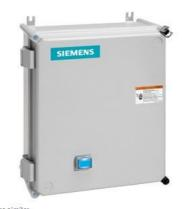
Non-reversing motor starter, Size 2 1/2, Three phase full voltage, Solidstate overload relay, OLR amp range 25-100A, 240V 50Hz / 277V 60Hz coil, Non-combination type, Enclosure type 4X fiberglass, Water/dust tight noncorrosive, Standard width enclosure
