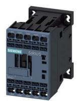
Coupling contactor relay, 2 NO + 2 NC, 24 V DC, 0.85 ... 1.85\* US, with integrated suppressor diode, Size S00, Spring-type terminal
