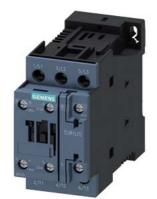
Power contactor, AC-3 38 A, 18.5 kW / 400 V 1 NO + 1 NC, 60 V DC 3-pole, size S0 screw terminals
