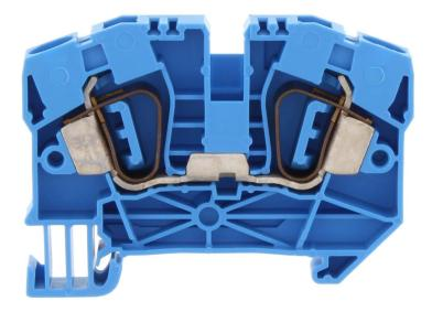
Ex feed-through terminal ATEX-certified, Tension-spring connection, Mounting type: Mounting rail TS 35/7.5, Rated cross-section: 6 mm<sup>2</sup>, Width: 8.1 mm, Colour: Blue
