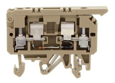
Fuse-disconnect terminal, Screw connection, Mounting type:Mounting rail TS 35/7.5 and TS 32, Rated cross-section: 4 mm², Width: 8 mm, Colour: Beige
