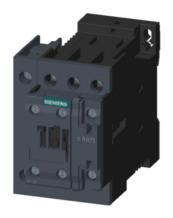
Contactor, AC-1, 35 A/400 V/40  $^{\circ}\text{C},$  S0, 4-pole, 220 V DC, 1 NO+1 NC, screw terminal
