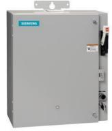
Pump control panel, Size 3, Three phase full voltage, Solid-state overload relay, OLR amp range 25-100A, 190-220/220-240V 50/60Hz coil, Standard type contactor, 200A fusible disconnect, 200A/250V fuse clip, HOA Sel Sw. <(>&<)> Start P.B., Enclosure NEMA type 3/3R, Weather proof outdoor use
