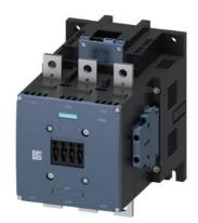
power contactor, AC-3 500 A, 250 kW / 400 V AC (50-60 Hz) / DC 200-277 V AC/DC auxiliary contacts 2 NO + 2 NC 3-pole, frame size S12 busbar connections drive: electronic with PLC interface 24 V DC screw terminal
