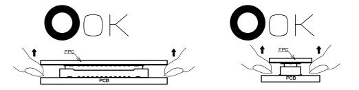
(2) IF THE CONNECTOR CANNOT BE UN-MATED PARALLEL IT CAN BE REMOVED DIAGONALLY FROM THE PITCH DIRECTION.
