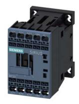
Power contactor, AC-3 9 A, 4 kW / 400 V 1 NO, 400 V AC, 50 / 60 Hz, 3-pole, Size S00 Spring-type terminal
