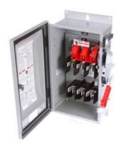
Siemens Low Voltage Circuit Protection Heavy Duty Safety Switches. Type: ENCLOSED, SAFETY SWITCH Std: UL V. Rating: 600V A. Rating: 60A Wattage: 3W No. Of Poles: 3P F. Rating: 60Hz Action: SINGLE THROW Material: 304SS Enclosure: TYPE 12. 2-3 point mounting holes. Insulation: YES O. Cycles: 10000 O. Temperature: (-20F-120F) AMBIENT TEMPERATURE Environmental Conditions: INDUSTRIAL
