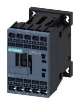
Power contactor, AC-3 12 A, 5.5 kW / 400 V 2 NO + 2 NC 24 V AC, 50/60 Hz 4-pole Size S00 Spring-type terminal
