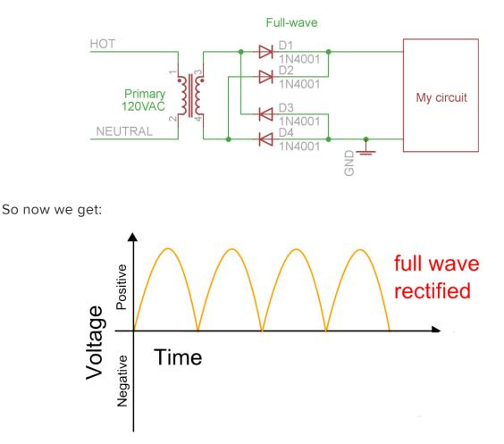
As you can see, there are twice as many humps - there isnt that "half the time, no voltage" thing going on. This means we can divide the calculated capacitor size to half of what it was in the previous.
