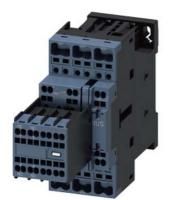
power contactor, AC-3 17 A, 7.5 kW / 400 V 2 NO + 2 NC, 220 V AC, 50 / 60 Hz, 3-pole, Size S0, Spring-type terminal Removable auxiliary switch
