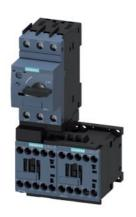
Load feeder fuseless, Reversing duty 400 V AC, Size S00 0.45...0.63 A 24 V DC screw terminal for installation on standard mounting rail (also fulfills type of coordination 1) Type of coordination 2, Iq = 150 kA 1 NC (contactor)
