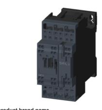
power contactor, AC-3 17 A, 7.5 kW / 400 V 1 NO + 1 NC, 220 V AC, 50 Hz, 240 V, 60 Hz, 3-pole, Size S0, Spring-type terminal
